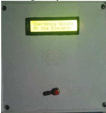
Figure 6a Shows hoe Emergency is displayed on the LED
