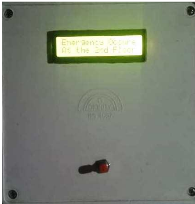
Figure 7a shows Emergency on the Second Floor
